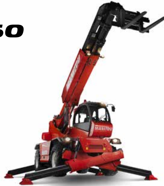
Rotation on lowered stabilizers with 1500 kg jib
