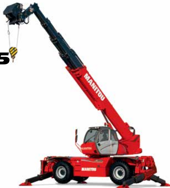
Rotation on lowered stabilizers with 3,300 lbs. (1500 kg) jib
